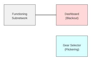
The gear selector remains operational because it resides on the lower-speed CAN-IHS bus (125kbps), while the dashboard modules use the high-speed CAN-C bus (500kbps). Water damage disproportionately affects CAN-C due to its higher impedance sensitivity.
